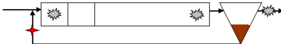
Figure 2: Layout of tracer experiment. Dosage in RAS and sampling at three points in the activated sludge tank and the effluent of the secondary clarifier
